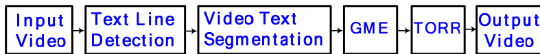
Fig. 6. Block diagram of the GM/LM based text occluded region recovery (TORR). The input video is with text occluded regions and the output video is with text occluded region recovery.
